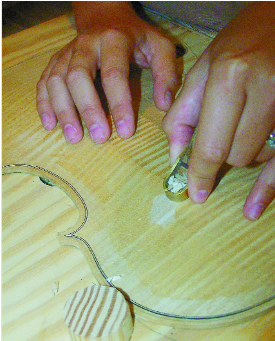
Using a tiny finger plane, Sonja St. John shapes the arched face of a violin she is making in her shop in Altus. St. John said it will take her a minimum of 200 hours to complete the delicate instrument.
